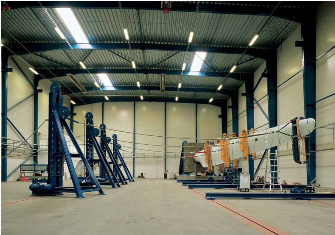
Figure 4: Full Scale Testing of Blades for Fatiguing
