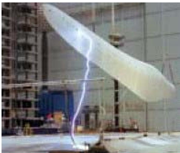
Figure 6 Full Scale Testing of Blade Lightning Protection
