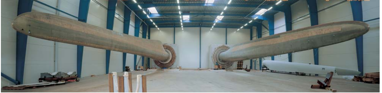
Figure 5: Full Scale Test Facilities for Blade Testing
